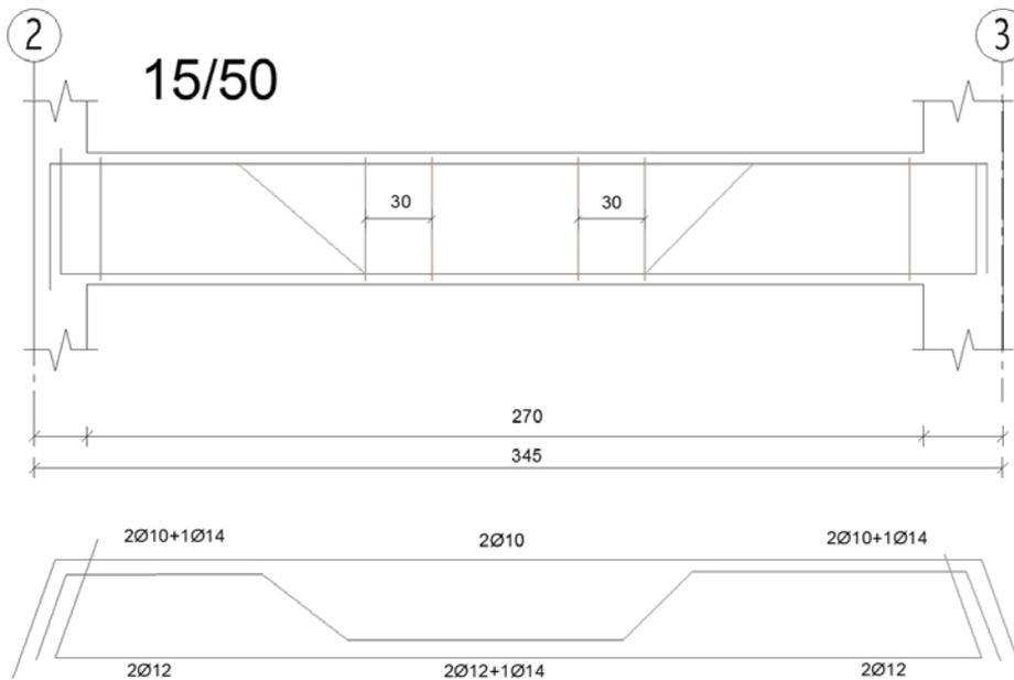
**Beam Reinforcement Details**
