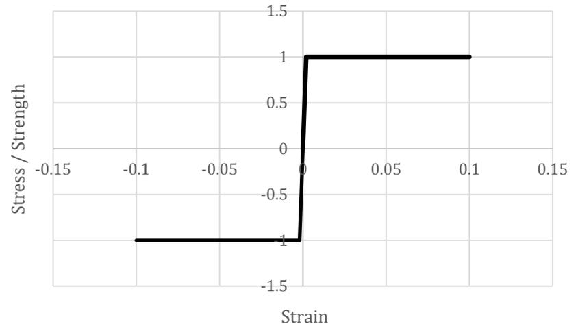
Nonlinear behavior of beams were modelled with moment-plastic rotation hinges.
